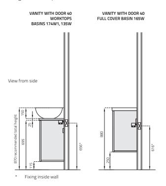
Included metal rail to be screwed on the wall. Below drawings show the centre of the mounting holes.
